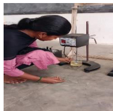
Figure 3: Bituminous softening test
